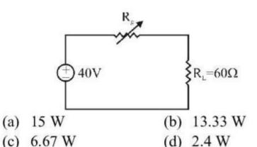
Determine the value of source impedance (in Ohms) for transmitting maximum power to the load in the circuit given below:
